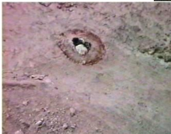
Figure 1 Sulfur balls of brimstone inside burned capsules, surrounded by burn rings embedded in ash.
